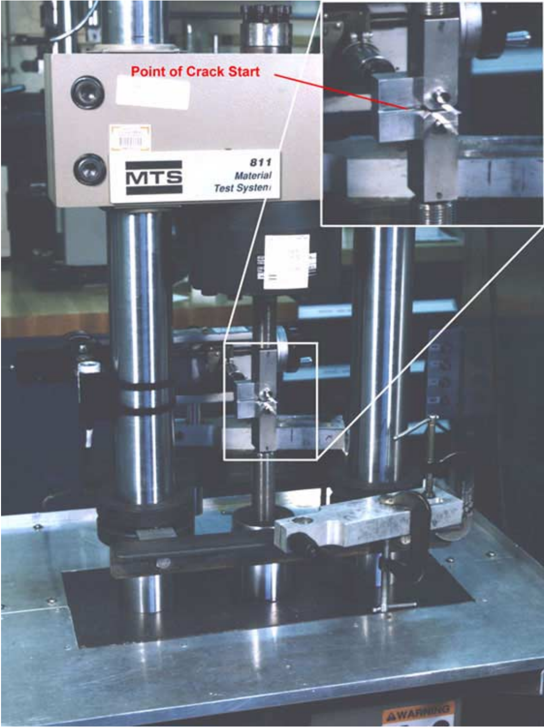
Exhibit 6-16 — Fracture Toughness Test Stand
